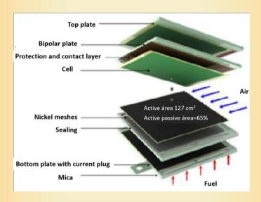
**Resumo:** Solid Oxygen Fuel Cells (SOFC) transform fuel and an oxidant directly into electrical energy and heat. They are since 20 y in the focus of numerous research activities due their high effectiveness. Typical applications range from mobile applications to small (5kW) and large (200kW) stationary applications for the production of electricity and heat.
